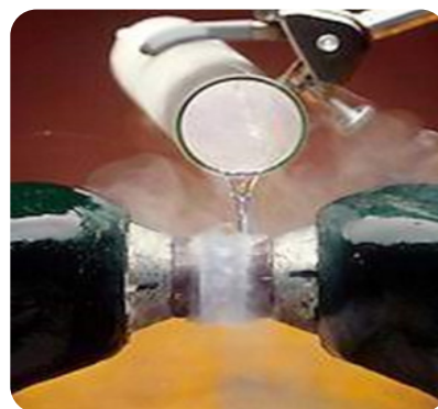
Liquid oxygen is attracted and gets suspended between the poles of a strong magnet
